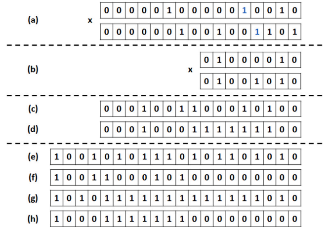
Fig. 4. Flow of the synergetic energy-efficient approximate multiplier. (a) Input value (b) Approximated input (c) Pre-shift operation result of DRUM (d) Pre-shift operation result of SEAM (e) Exact result (613,738 10 ) (f) Result of DRUM (616,224 10 ) (g) Result of AWTM (720,890 10 ) (h) Result of SEAM (622,496 10 ).
